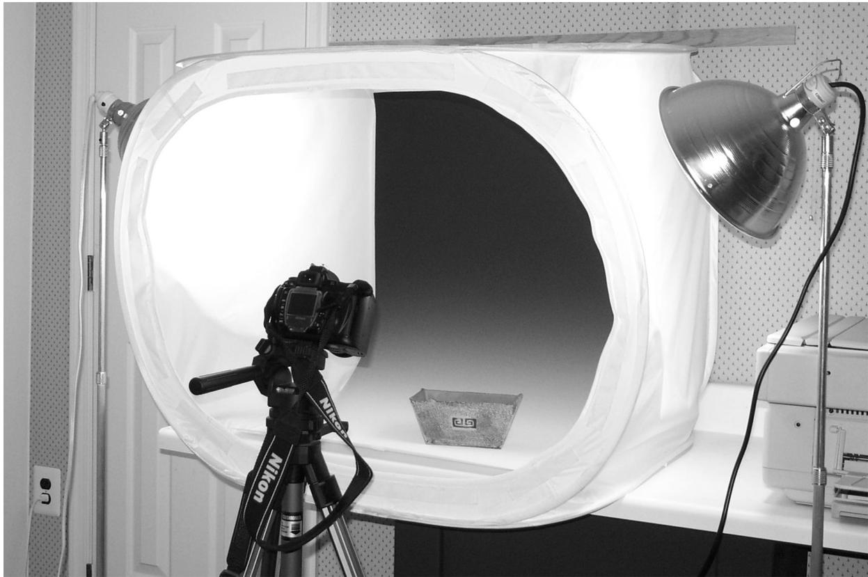
Light tents are made from tightly woven white nylon fabric. The nylon fabric softens and diffuses the light which is directed at the work through the fabric. Alternatives include soft boxes with an electronic flash inside (what I used to use), reflective umbrellas, and two or three other combinations of a light source combined with some means of softening or diffusing the light.
